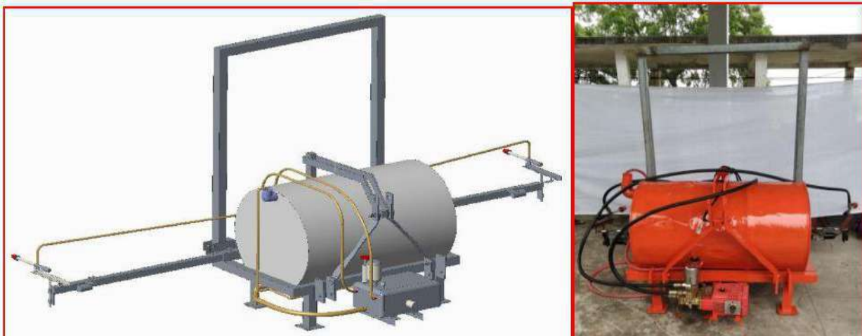
Fig.3 Developed low HP tractor operated wiper sprayer
