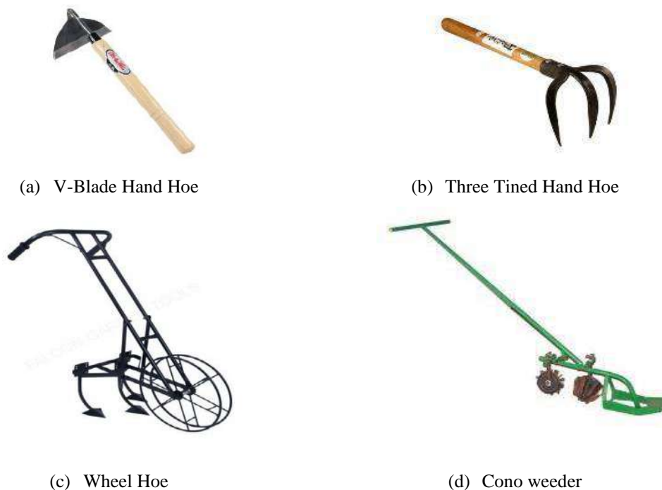
Fig.4 Manual operated weeding tools
