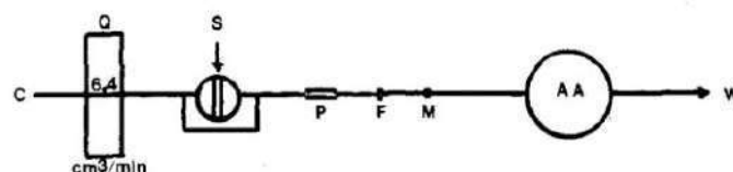
Fig.1: Illustrate the schematic diagram of FI manifold associated to FIA-AAS assessment of free \text{CN}^- ; C, carrier; Q, flow rate ( \text{cm}^3/\text{min} ); S, point of injection; P, packed column; F, filter; M, the connection point to the nebulizer; AA, detector; W, waste (Haj-Hussein et al., 1986).
