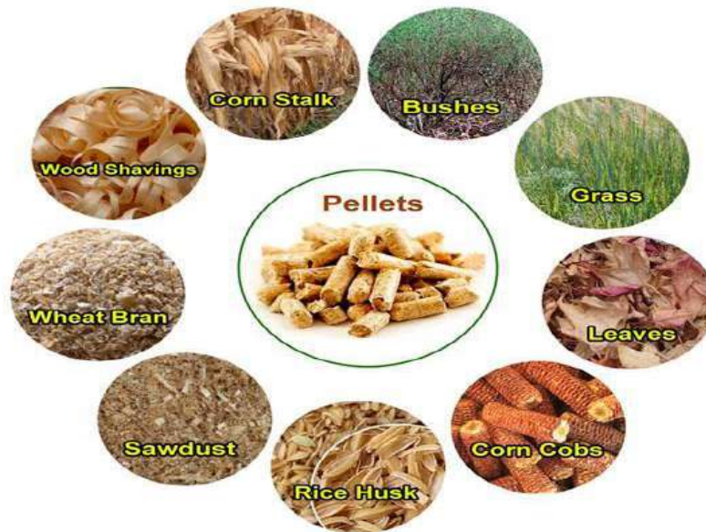
Fig.1: Biomass sources for pelletizing (Kiss and Alexa, 2014).
