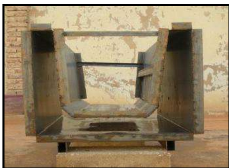
Plate (1) Fabricated inner steel form section
