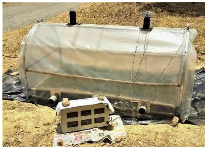
Fig. 4 Drying of mint leaves in LCSD
